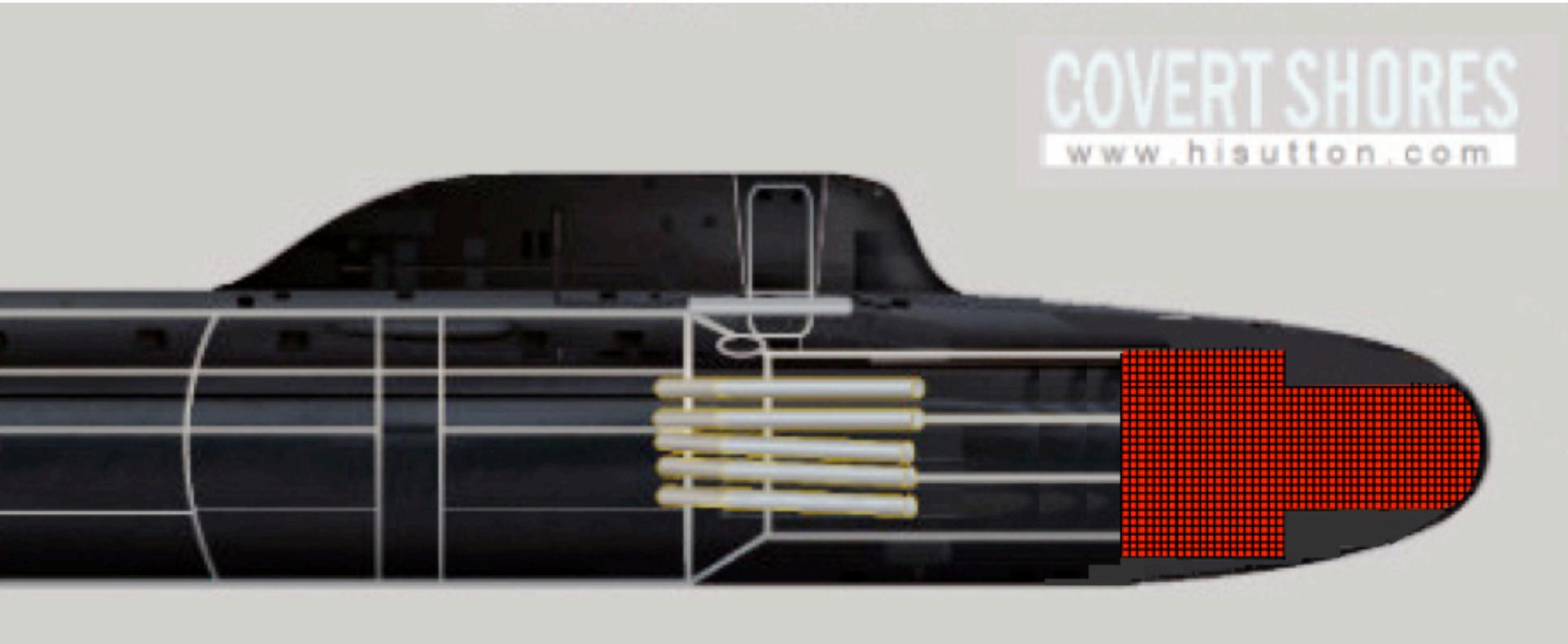
Replacing the separate sphere and flank arrays with an integrated conformal/flank array design allows the Russians to reduce the size of the bow while at the same time increasing the the effective area of the main hull arrays.
