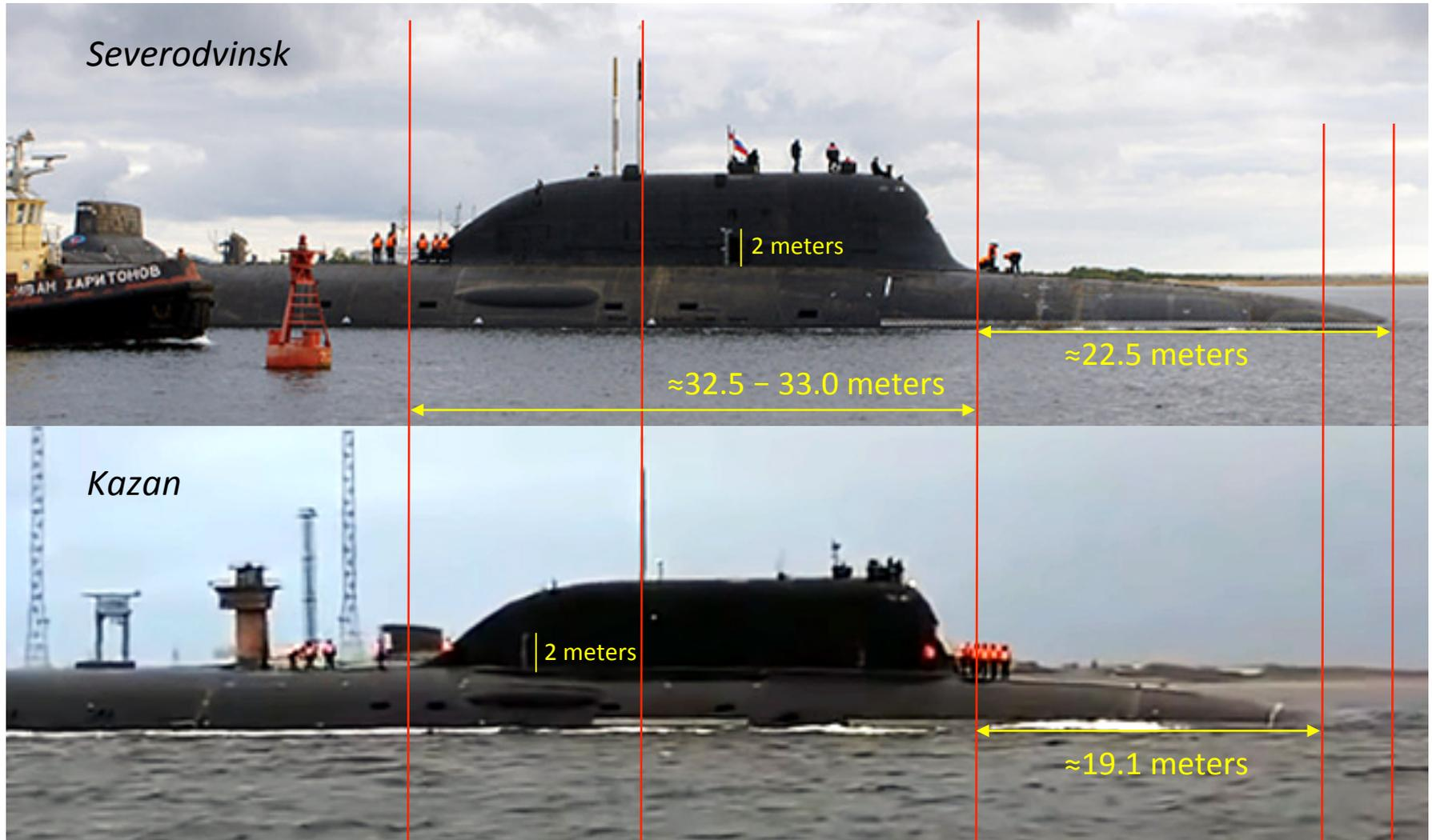
A comparison of the two boats from a nearly identical aspect, with the sail draft markings in view, shows the bow of *Kazan* is about 3.5 meters shorter than *Severodvinsk*, above the waterline. The sail length on both submarines is essentially identical at 32.5 - 33.0 meters.
