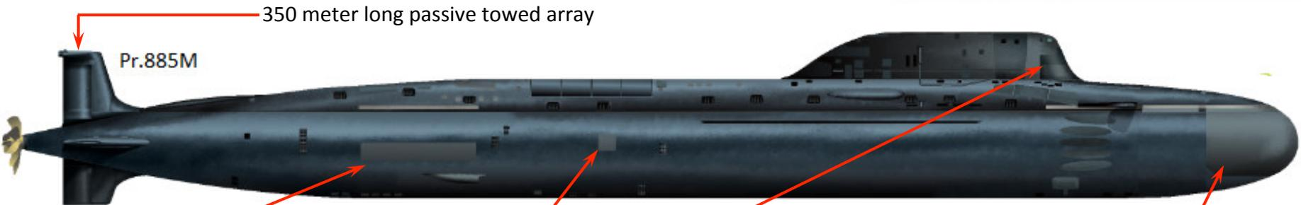
350 meter long passive towed array
