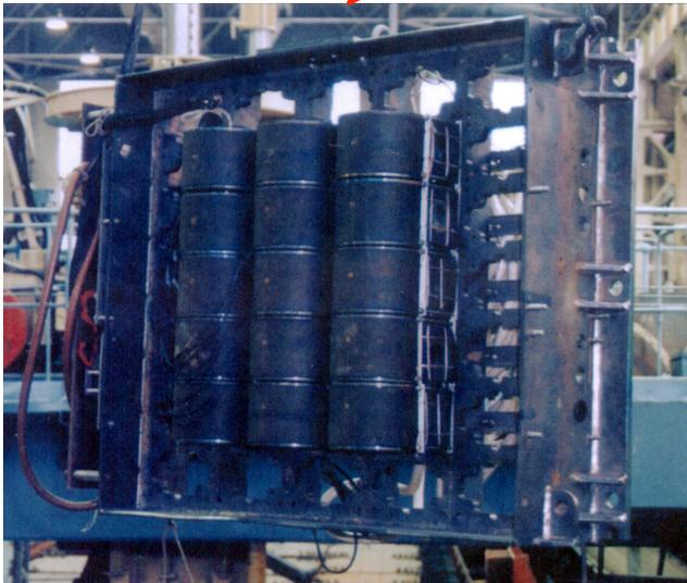
Integrated passive conformal and flank arrays
