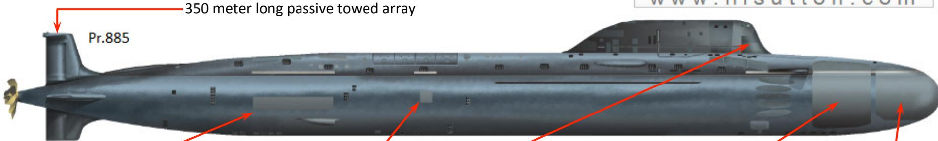
350 meter long passive towed array
